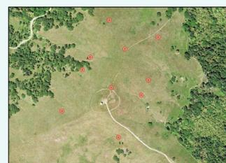
Figure 4. Ground control points for the study area. Data was collected with a Trimble Geoexplorer 6000.
