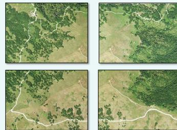
Figure 1. Images captured with a sUAS can be stitched together into high-resolution mosaics.
